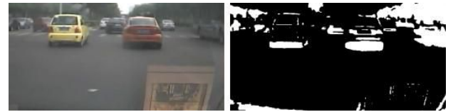
Figure 3. Shadow Segmentation in the Traffic Scene
