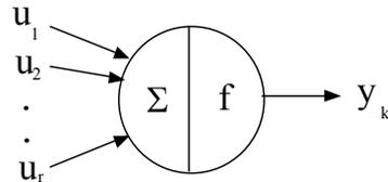
Fig.3 Neuronal architecture with r inputs
