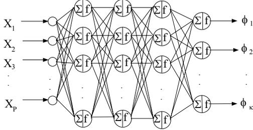
Fig.1 Architecture of revised GMDH-type neural networks.
