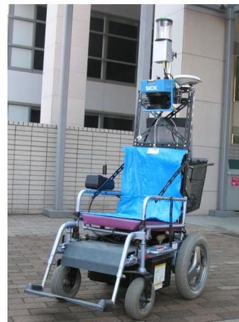
Fig. 1. Configuration of proposed human following intelligent wheelchair
