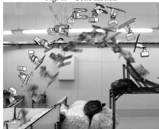
Fig. 20 Sequential pictures of the performing robot in the flight experiment in side view
