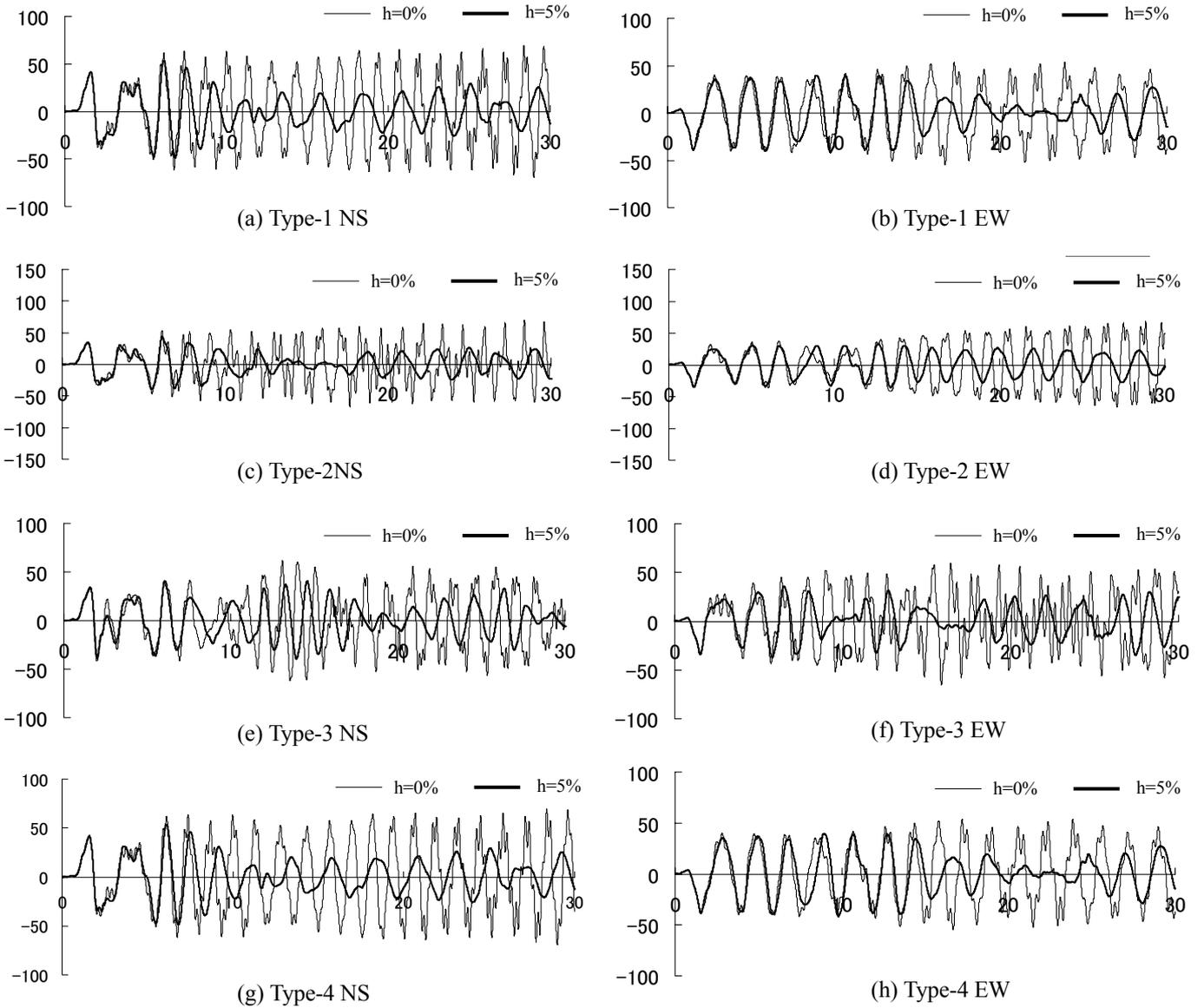
Figure 7. Influence of damping to nonlinear response with nonperiodic and high frequency component.
