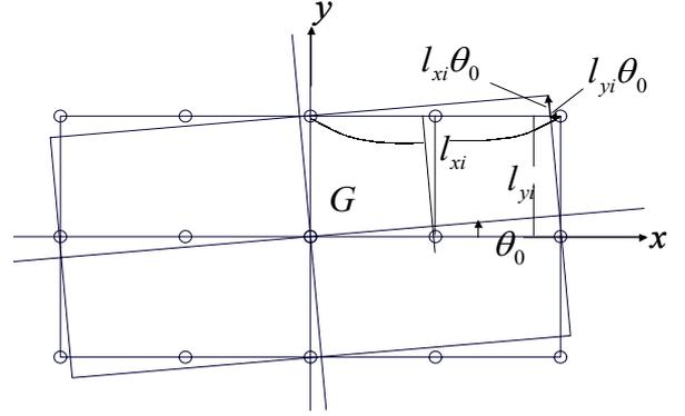
Figure 3. Rotation of a rigid base and horizontal displacements of isolators.
