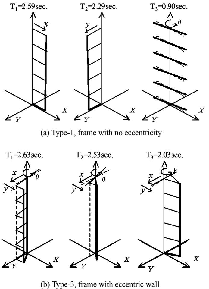
Figure 6. Natural period and base condition of structure.
