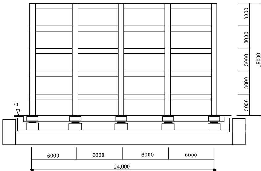
Figure 5. Reinforced concrete framework sustained by seismic isolators.
